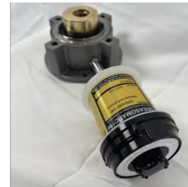
Lubricate thrust bearings
